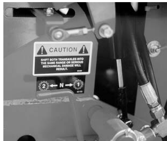
Photo 10 - Neutral Linkage Adjustment
