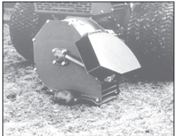
Photo 2 Discharge Chute Left Airflow Position
